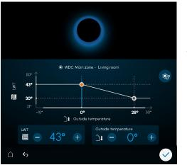
Thanks to the Weather Dependent Curve - optimal comfort and high efficiency with automatically determined desired temperature.
